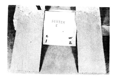
System E After Accelerated Weathering FIGURE 16
