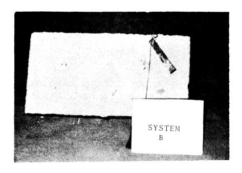
System B After Abrasion Test FIGURE 8
