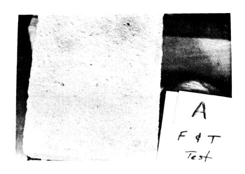
System A After Freeze and Thaw Test FIGURE 18
