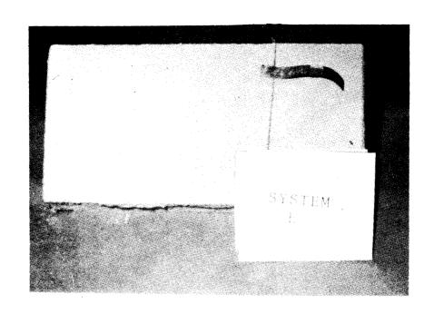
System E After Abrasion Test FIGURE 11
