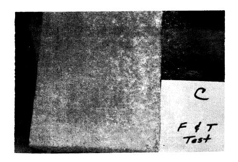
System C After Freeze and Thaw Test FIGURE 20
